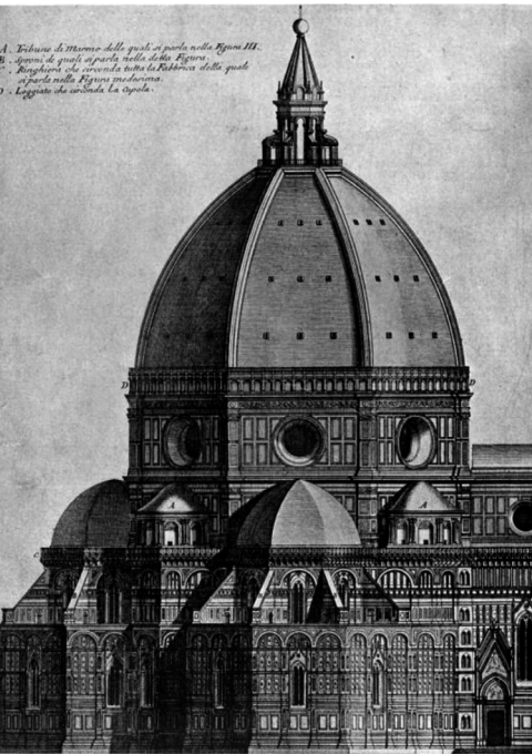
S. MARIA DEL FIORE, FLORENCE Elevation of dome and substructure. (From Sgrilli)
